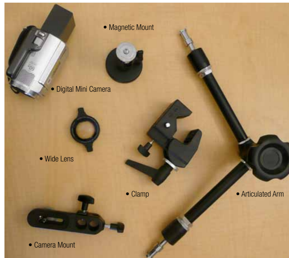
Figure 4a - Mounting equipment with camera
