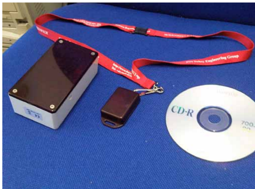
Figure 5 - IR field generating beacon (top) and IR logging tag (bottom)
