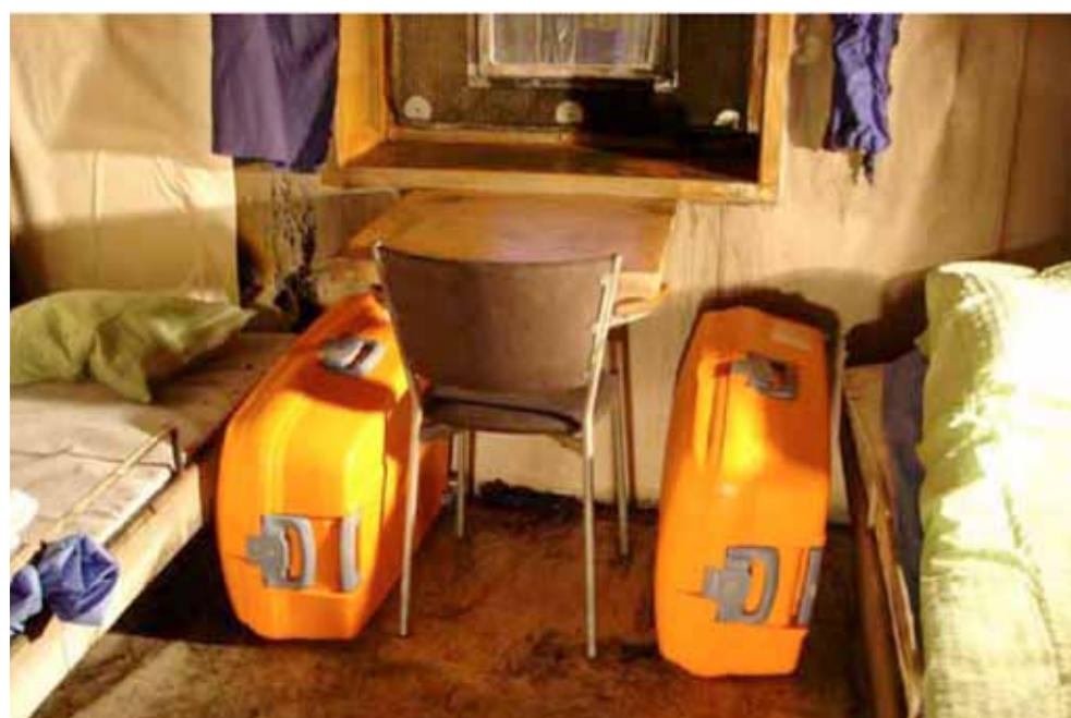
Figure 1 - Cabin material in SP cabin fire test 1: Figure reproduced from Arvidson, M., Axelsson, J., and Hertzberg, T. (2008) Large-scale fire tests in a passenger cabin, SP Report 2008:33, SP Technical Research Institute of Sweden.
